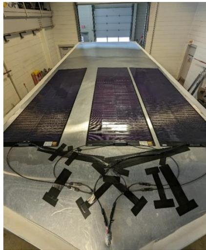
Parks Services Team is excited to announce they completed their first solar powered trailer! This trailer is upfitted with 600W of solar panels and a power bank to charge the batteries that power our landscaping equipment. The trailer will be used this summer for our EGO lawn mowing and EV Gravely zero turn mowing equipment. Staff will continue to track the trailers functionality this spring and summer.
